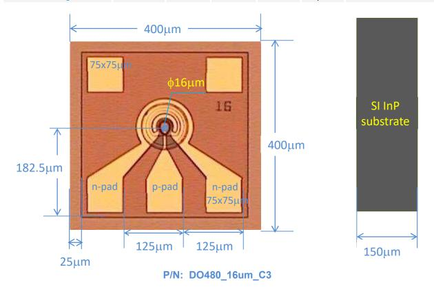
Attention: InP brittle material and electrostatic sensitive device, observe precaution for handling.
